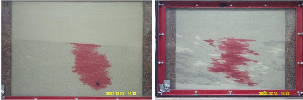
The behavior of NAPL in heterogeneous porous materials. Pictures show a light non-aqueous phase liquid (red spill) in a water saturated layered medium with an inclined interface (left) and highly heterogeneous medium with random distribution of heterogeneities (right), respectively (provided by CESEP, Colorado School of Mines).
